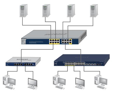
Figure 4. Backbone switching
